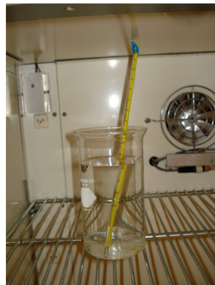
Figure 3. Glass thermometers are used to verify the inside temperature of each incubator.
