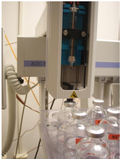
Figure 17: Checking the position of the needle. Make sure the needle is centered over the rubber or it may break when it hits the
